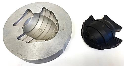
**Figure 1.** Mold manufactured by EDM (left) and EDM electrode (right).
