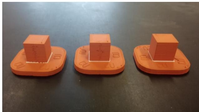
**Figure 4.** Cubic test samples manufactured by ADAM technology.
