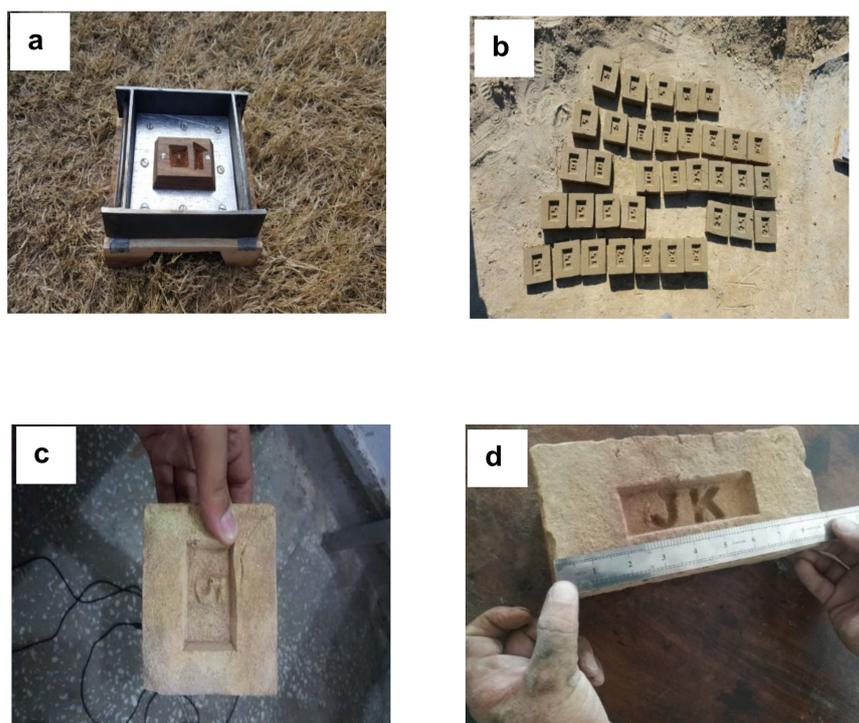
**Figure 3.** (a) Mold of radiation specimen. (b) Radiation brick specimen preparation. (c) Radiation brick specimen. (d) Normal brick specimen.
