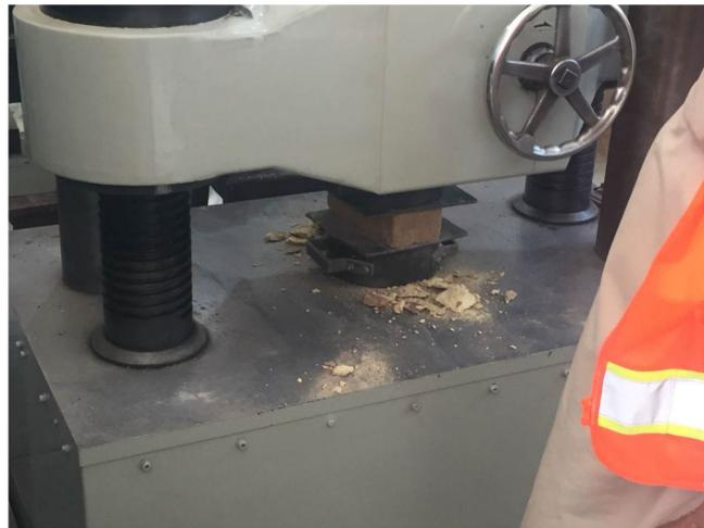
**Figure 4.** Compressive strength in universal testing machine.
