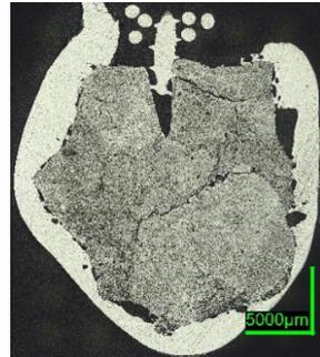
**Figure 11.** Digital microscope images of the HBI-ULC-2-1 sample, dipped into ULC.
