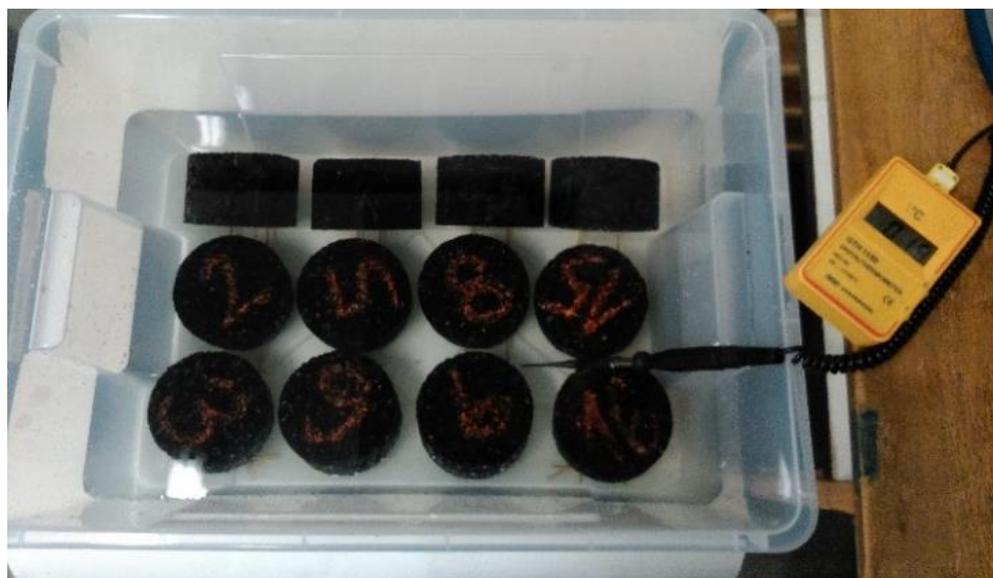
**Figure 1.** Samples in distilled water before freeze–thaw cycles (Photo: Authors).
