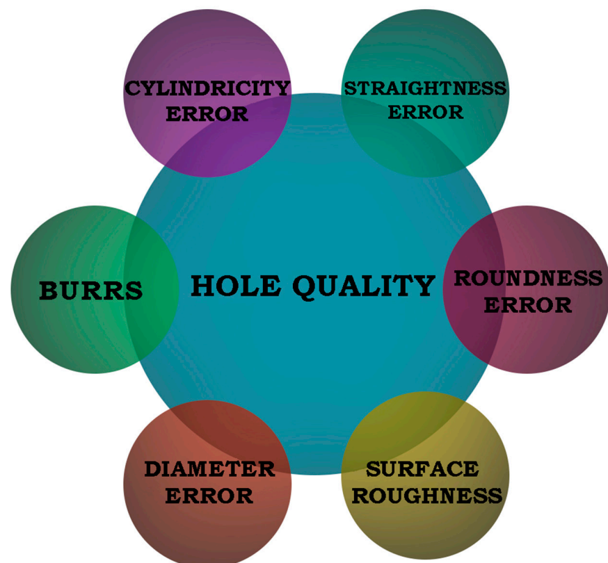
Figure 3. Parameters describing the hole quality.
