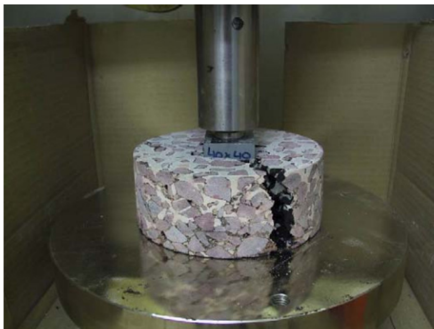
Figure 4. Test setup of indentation strength [57].
