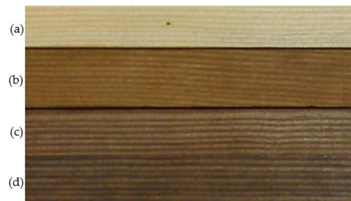
**Figure 1.** Sample surface—control (a) and heat-treated wood (constant temperature of heat treatment—220 °C) at a heat treatment duration of 1 h (b); 2 h (c); 8 h (d).
