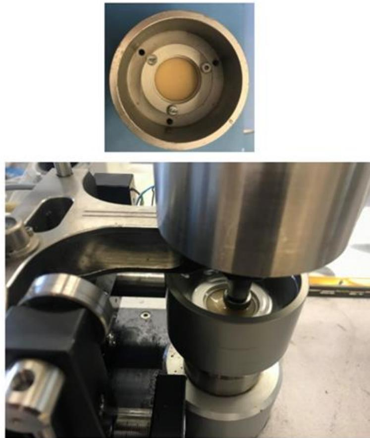
**Figure 2.** The pin-on-disc test setup used for the wear resistance study.
