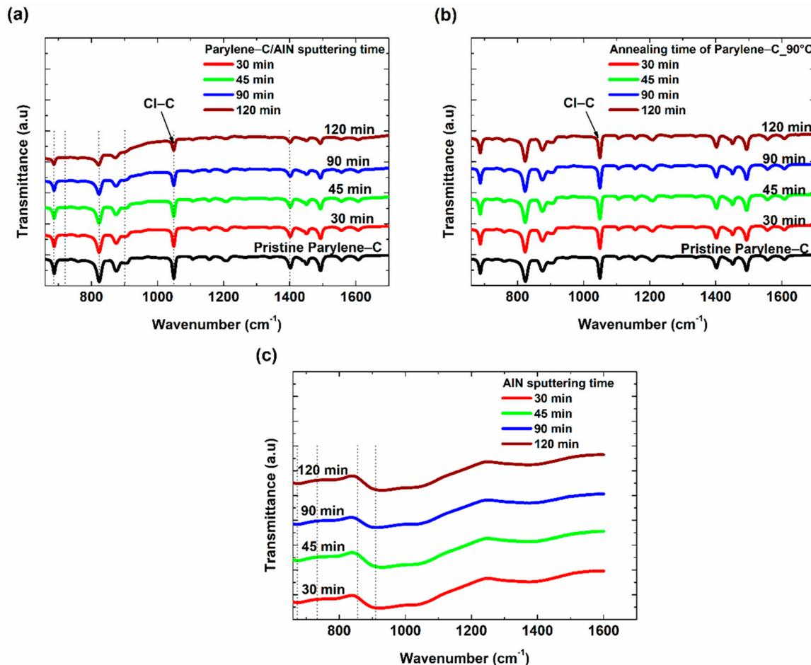
**Figure 3.** FTIR spectra. (a) Pristine parylene-C and parylene-C/AlN samples. (b) 90 °C Annealed parylene-C. (c) AlN samples, with respect to sputtering time.
