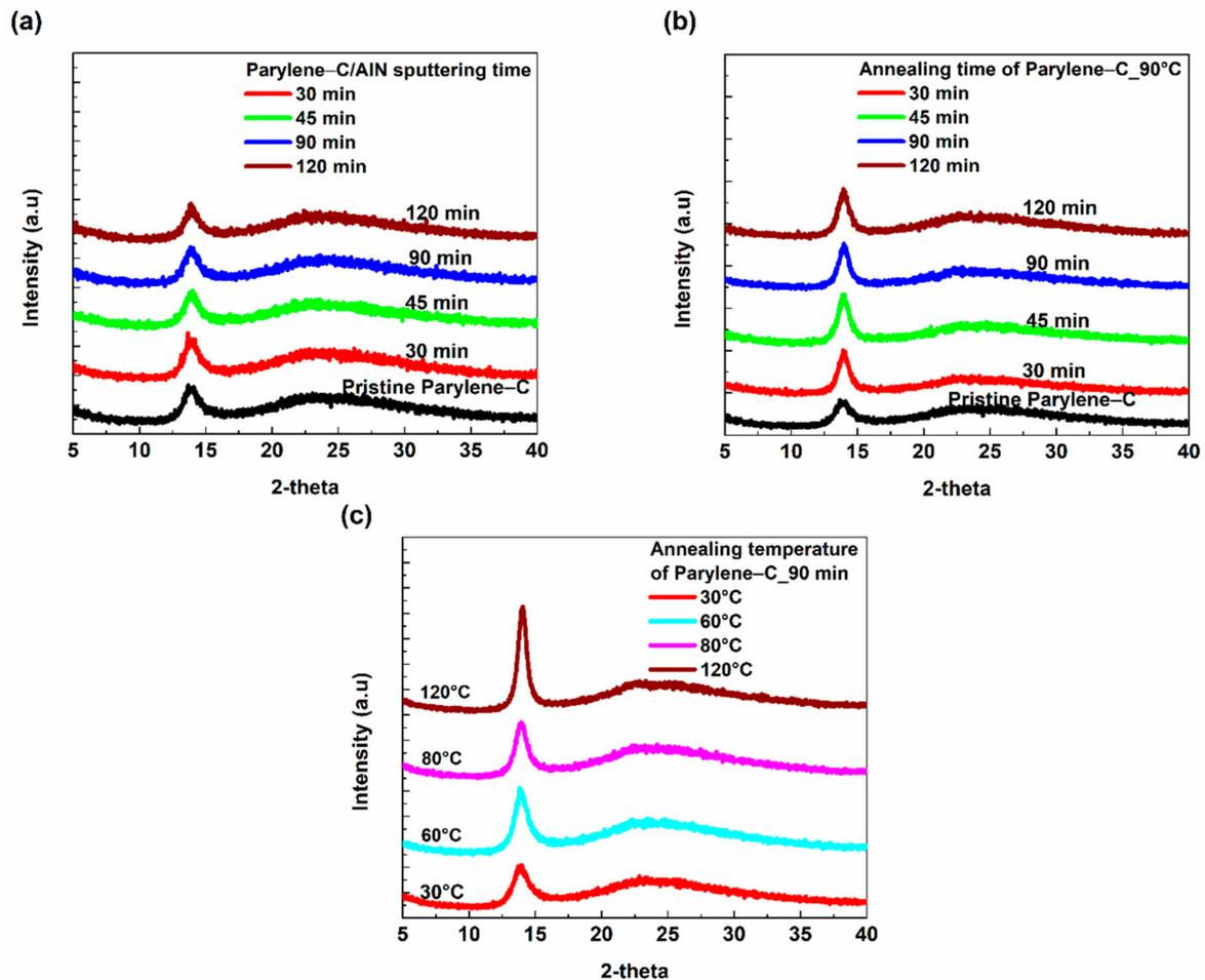
**Figure 5.** XRD patterns. (a) Pristine parylene-C and parylene-C/AlN samples. (b) 90 °C annealed parylene-C from 30–120 min. (c) 30, 60, 80 and 120 °C annealed parylene-C for 90 min.
