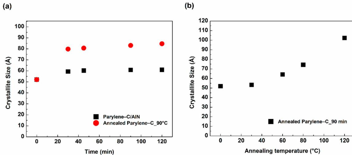
**Figure 6.** (a) Crystallite sizes of parylene-C/AlN and 90 °C annealed parylene-C with respect to sputtering and annealing time, respectively. (b) Crystallite sizes of 30, 60, 80 and 120 °C annealed parylene-C for 90 min.
