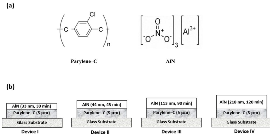
**Figure 1.** (a) The chemical structure of Parylene-C and AlN. (b) The schematic structures of AlN deposited on Parylene-C with respect to sputtering time.
