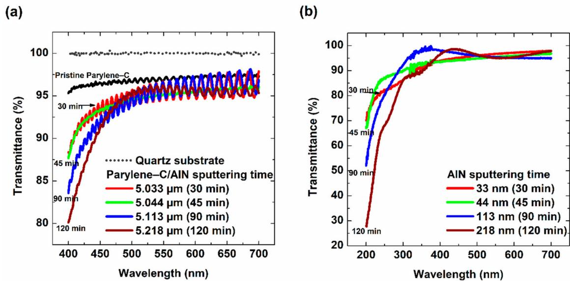
**Figure 2.** The transmittance spectra. (a) Quartz substrate (reference), pristine parylene-C and parylene-C/AlN samples, in the visible range. (b) Quartz substrate (reference) and AlN samples with respect to sputtering time.
