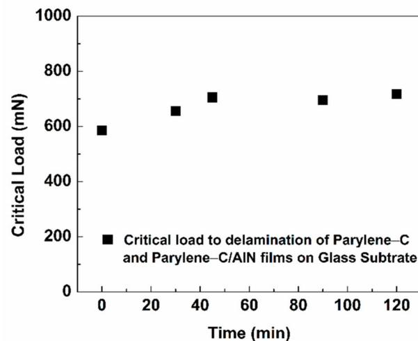
**Figure 7.** The critical load to delamination comparison of pristine parylene-C and parylene-C/AlN films, with respect to sputtering time.
