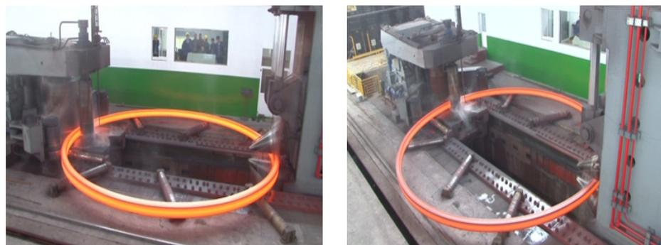
**Figure 17.** Experiment of RARR process for a super-large ring.
