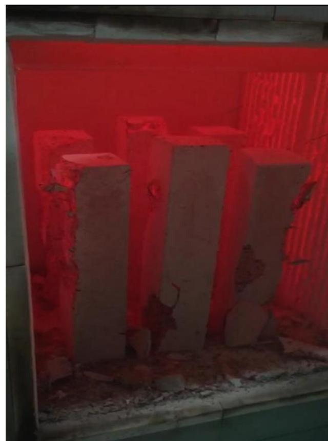
**Figure 11.** Samples that spalled inside the oven.
