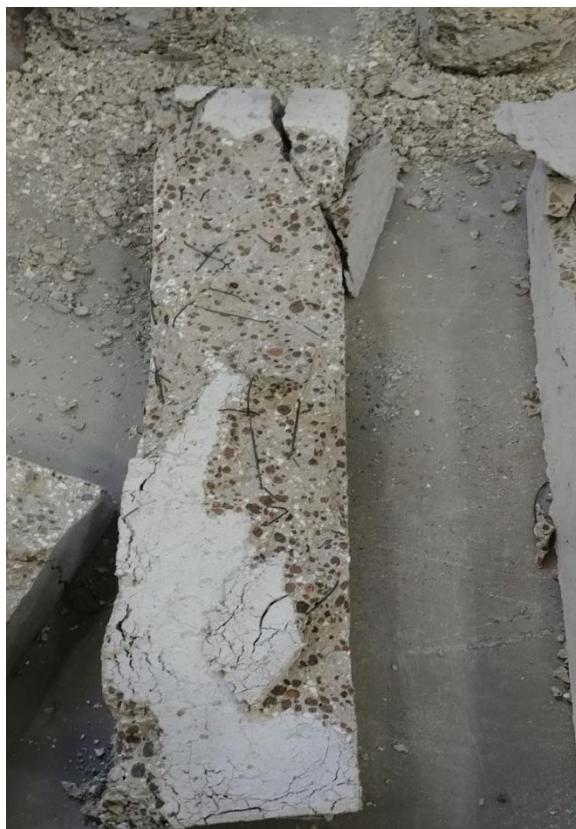
**Figure 22.** Spalled samples after temperature loading with 800 °C.
