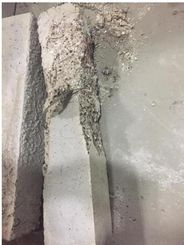
Figure 12. Deteriorated surface of 500 °C sample after water cooling.
