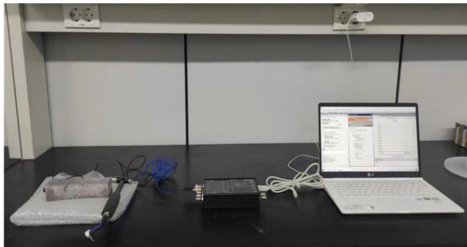
**Figure 2.** A picture of the damping ratio test setup.
