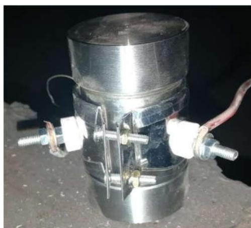
**Figure 2.** The assembly diagram for slow cook-off test.
