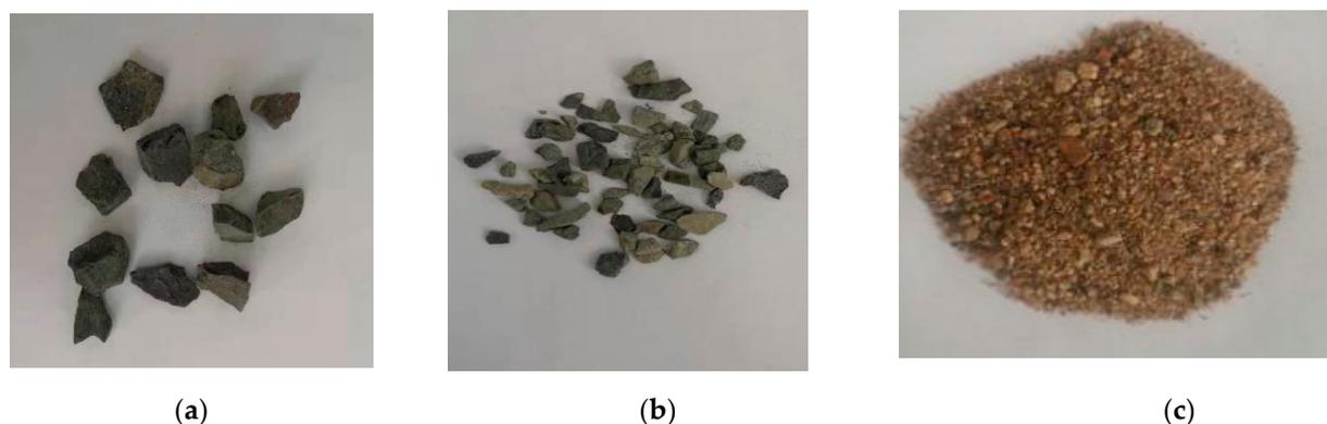
**Figure 1.** Particle size distribution. (a) Particle size 4.75–9.5 mm. (b) Particle size 9.5 mm–19 mm. (c) Medium sand.
