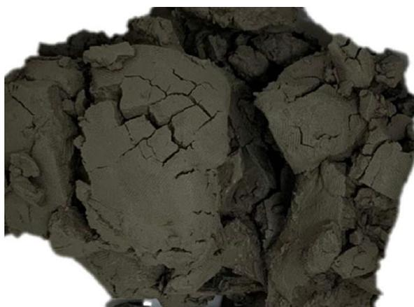
**Figure 3.** Concrete sludge waste (CSW) immediately after dehydration with moisture content of 40%.**Table 3.** Factors and levels.
