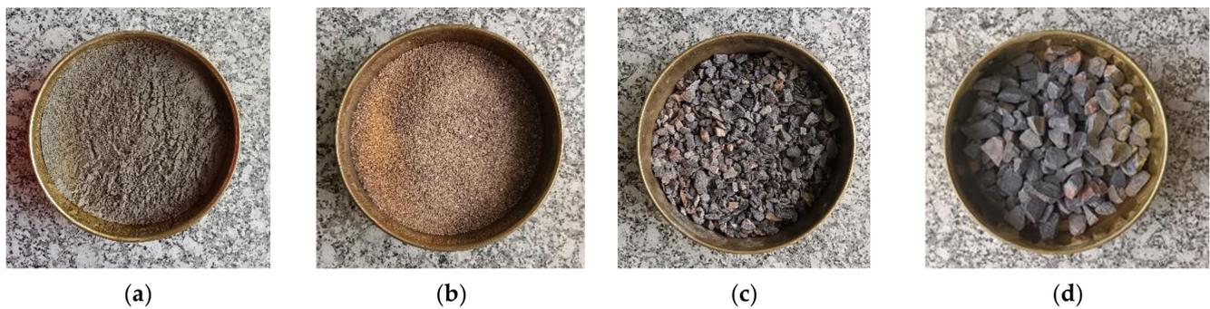
**Figure 1.** (a) Commercial cement; (b) river sand; (c) natural coarse aggregates (NCA)—10 mm; (d) natural coarse aggregates (NCA)—20 mm.
