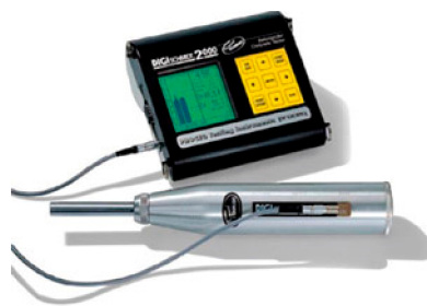
Figure 6. SCHMIDT rebound hammer test apparatus.
