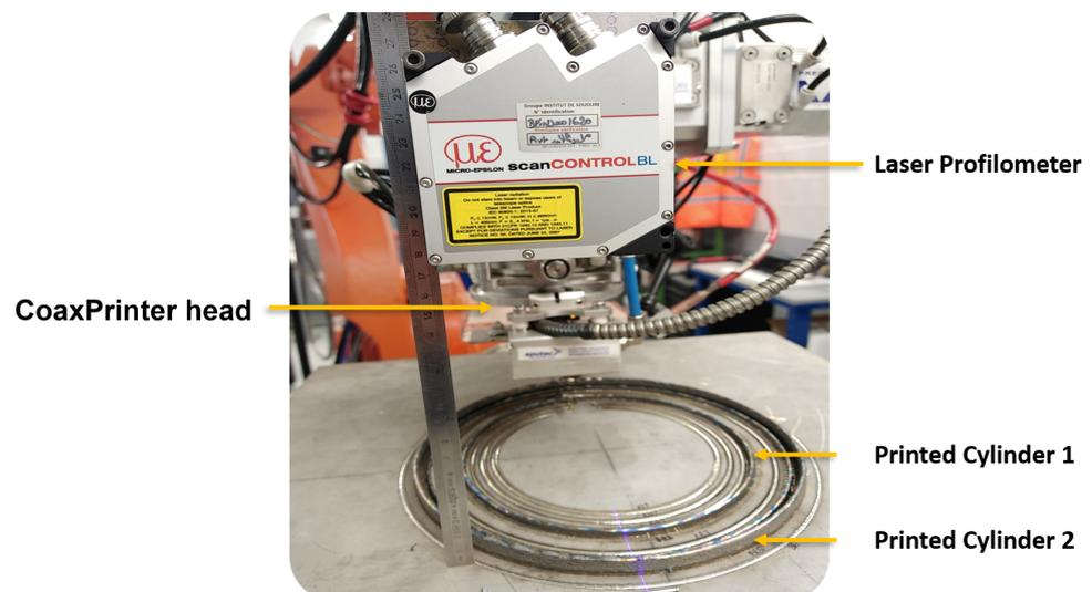
**Figure 7.** Profilometer set-up for data acquisition.
