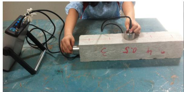
**Figure 5.** Semi-direct UPV measurement.
