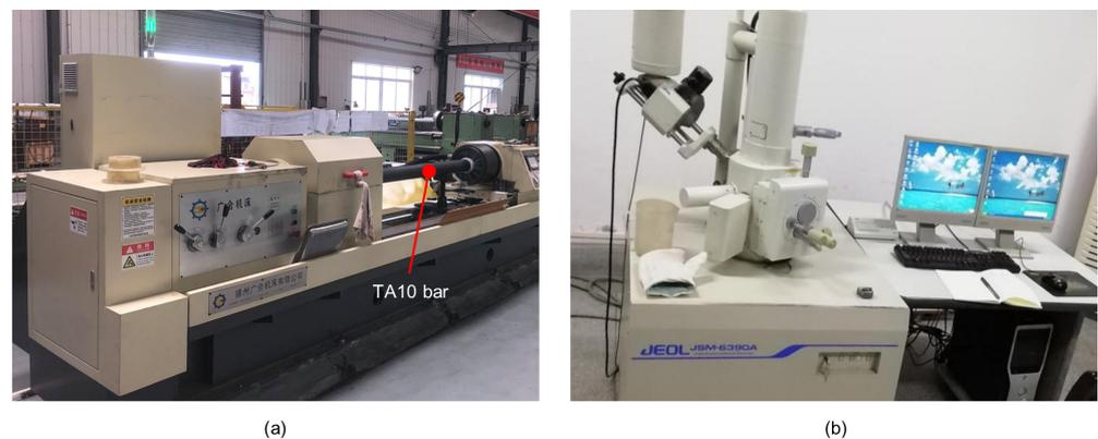
**Figure 2.** Processing environment and experiment equipment. (a) T2120G deep-hole drilling and boring machine (Dezhou, China); (b) scanning electron microscope JSM-6390A (Akishima, Japan).
