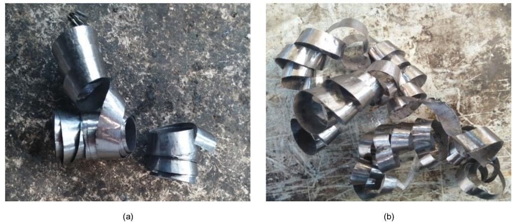
**Figure 5.** Chip morphologies. (a) Short spiral chips. (b) Long coiled chips.
