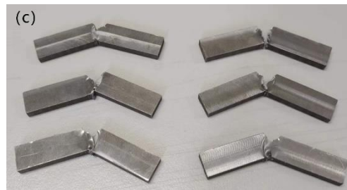
Figure 4. Schematic diagram of tensile and impact sampling (a) Sampling location; (b) Tensile test specimen; (c) Impact specimen.
