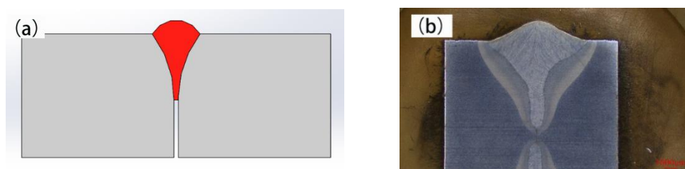
Figure 2. Welding diagram of I-groove joint (a) Welding diagram (b) Macroscopic.
