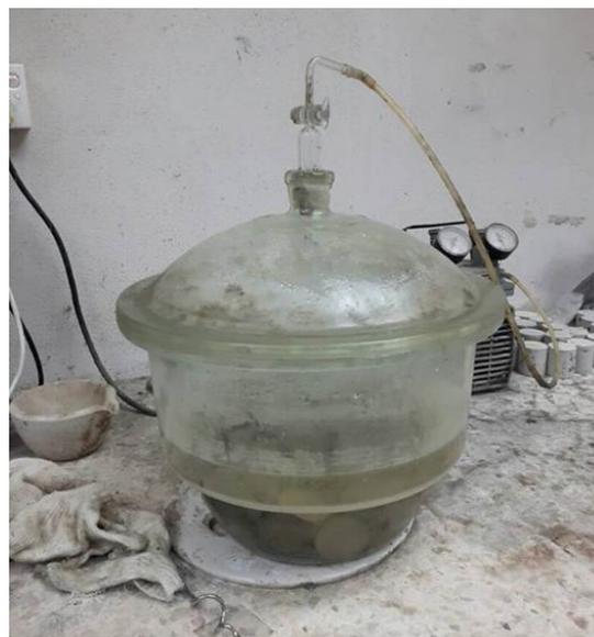
**Figure 5.** Porosity test via vacuum saturation method.
