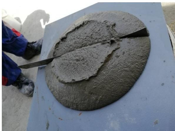
**Figure 3.** Slump test of fresh LFC.
