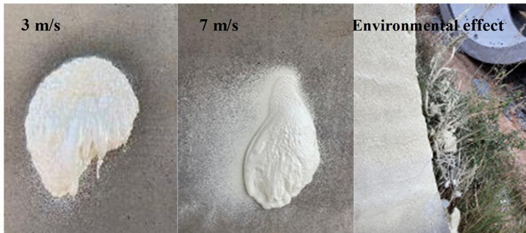
**Figure 7.** Polymer spraying performance at different  $v_{wind}$ .
