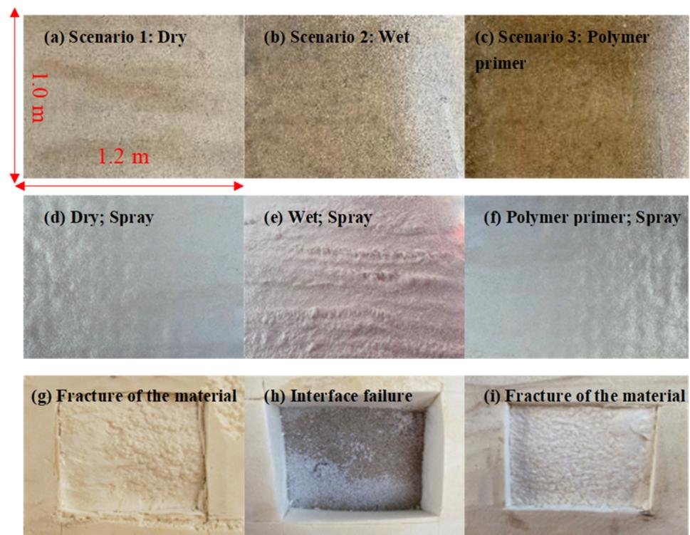
**Figure 6.** Three scenarios, spraying performance and adhesive strength tests under three scenarios: (a–c) for Scenarios 1~3; (d,g) for Scenario 1; (e,h) for Scenario 2; (f,i) for Scenario 3.
