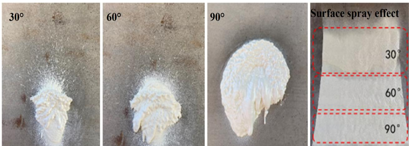
**Figure 11.** Spraying performance at different  $\theta_{spray}$ .
