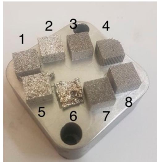
**Figure 9.** Image of samples manufactured by the SLM process from 1CP alloy powder (numbers 1–8 denotes the building mode of Table 7).
