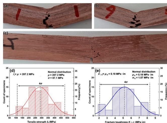
**Figure 5.** (a–c) Side views of the failed samples, and the normal distribution of the tensile strength (d) and fracture toughness (e) of BW.
