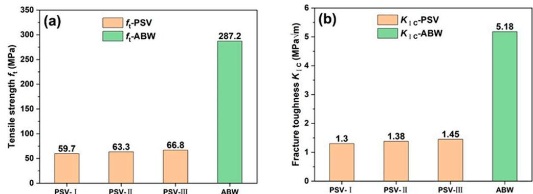
**Figure 7.** Comparison of the tensile strength (a) and fracture toughness (b) of PSV and BW.
