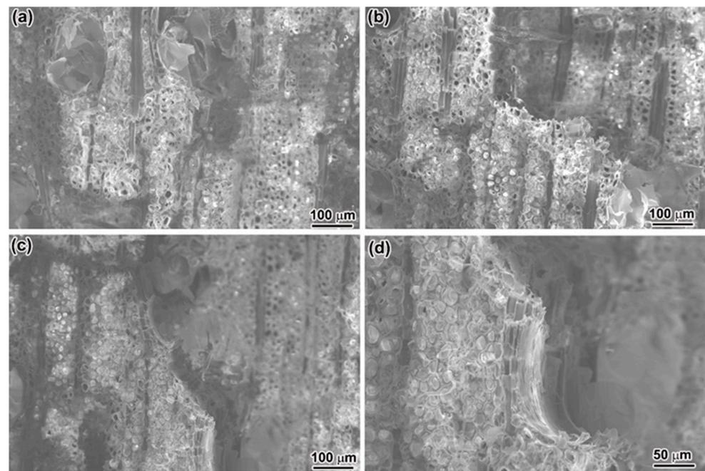
**Figure 6.** SEM images of fractured vessels (a,b), cracks propagate from one vessel to the adjacent vessel (c), and the magnified images of one fractured vessel (d) in failed BW samples.
