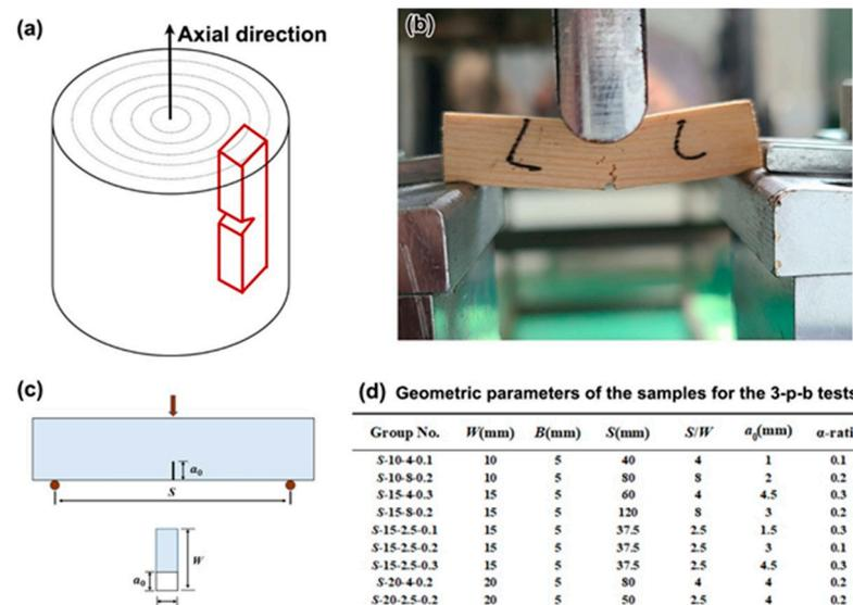
**Figure 1.** Schematic diagram for the preparation of samples (a) and the actual loading device (b) for 3-p-b tests, and schematic diagram of the dimension of samples (c), together with the geometric parameters (listed in Table) (d) for the 3-p-b tests.
