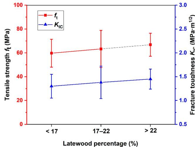
**Figure 4.** Distribution of the tensile strength and fracture toughness with different volume percentages of the latewood of PSV.
