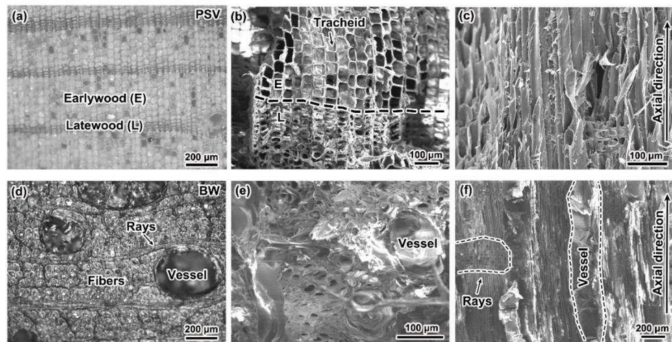
**Figure 2.** Microstructures on the transversal plane (a,b) and longitudinal plane (c) of PSV, and transversal plane (d,e) and longitudinal plane (f) of BW.
