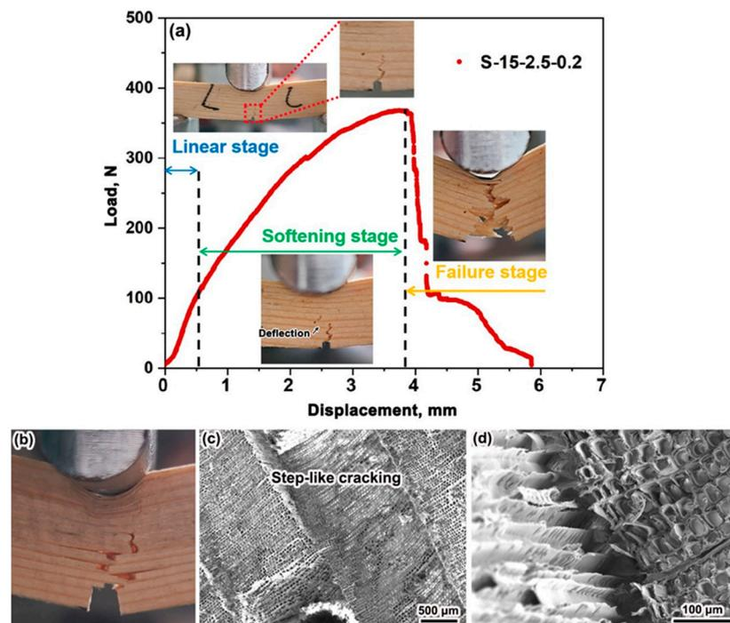
**Figure 3.** Simplified three-stage quasi-brittle fracture process (a), the side view under testing (b), and detailed morphologies of the fracture surface (c,d) of the PSV sample.
