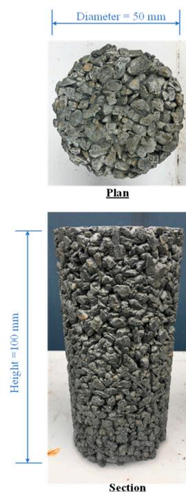
**Figure 5.** CFG specimen.
