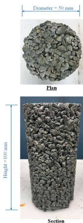
**Figure 5.** CFG specimen.
