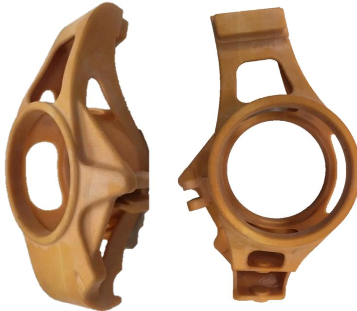
**Figure 6.** The upright model printed by the BJ (binder jetting) method.
