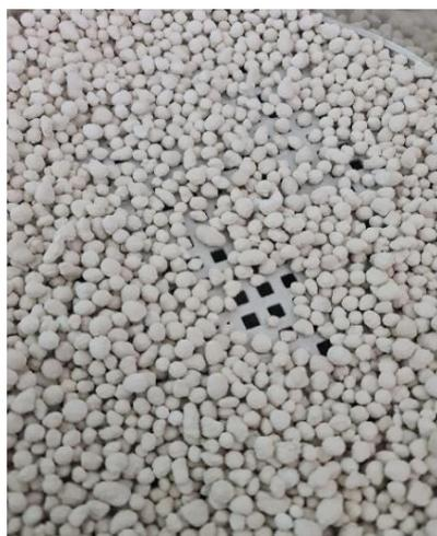
**Figure 1.** Gypsum granules during sieving through successive sieves.
