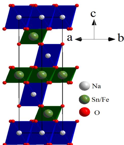
**Figure 5.** Rhombohedral crystal structure of  $\text{Na}_{0.8}\text{Fe}_{0.8}\text{Sn}_{0.2}\text{O}_2$ . Red, white, and green spheres represent oxygen, sodium, and Fe/Sn atoms, respectively.
