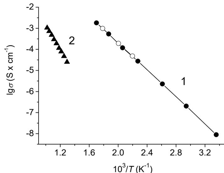
**Figure 8.** Temperature dependences of electroconductivity for  $\text{Na}_{0.8}\text{Fe}_{0.8}\text{Sn}_{0.2}\text{O}_2$ : (1) total conductivity; solid circles—heating, open circles—cooling; (2) electronic conductivity.
