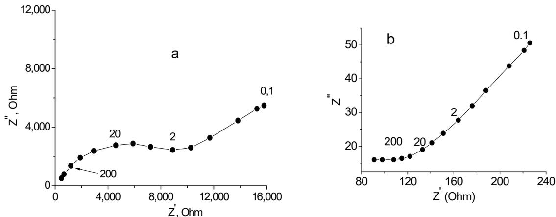
**Figure 7.** Impedance spectra for Ag |  $\text{Na}_{0.8}\text{Fe}_{0.8}\text{Sn}_{0.2}\text{O}_2$  | Ag cell: (a) 182; (b) 368 °C. Numbers above the curves represent frequencies (kHz).
