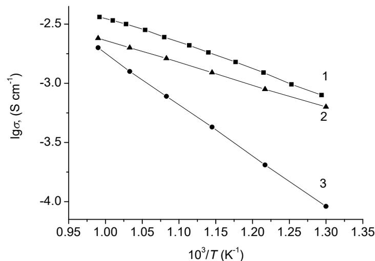
**Figure 6.** Temperature dependences of  $\text{NaFeO}_2$  conductivity: (1) total; (2) ionic; (3) electronic conductivity.
