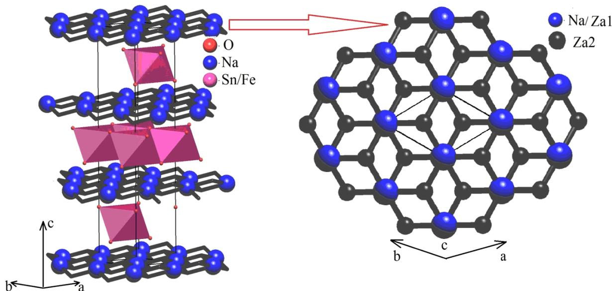
**Figure 9.** Migration map (left) and 2D migration layer (right) for rhombohedral  $\text{Na}_{0.8}\text{Fe}_{0.8}\text{Sn}_{0.2}\text{O}_2$ ; large blue spheres— $\text{Na}^+$  ions coincide with Za1 significant voids, black spheres—Za2 significant voids in the center of the vacant tetrahedral interstitial site, and black lines—elementary migration channels, Sn/FeO6 octahedra are pink.
