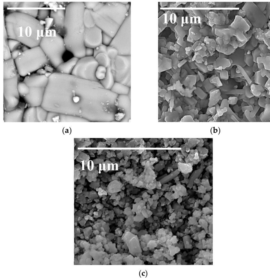
**Figure 2.** SEM image of the surface of the sintered  $\text{Na}_{0.8}\text{Fe}_{0.8}\text{Sn}_{0.2}\text{O}_2$  pellets in the  $\text{NaFeO}_2$ – $\text{SnO}_2$  system: (a) 5; (b) 20 ( $\text{Na}_{0.8}\text{Fe}_{0.8}\text{Sn}_{0.2}\text{O}_2$ ); (c) 35 mol.%  $\text{SnO}_2$ .
