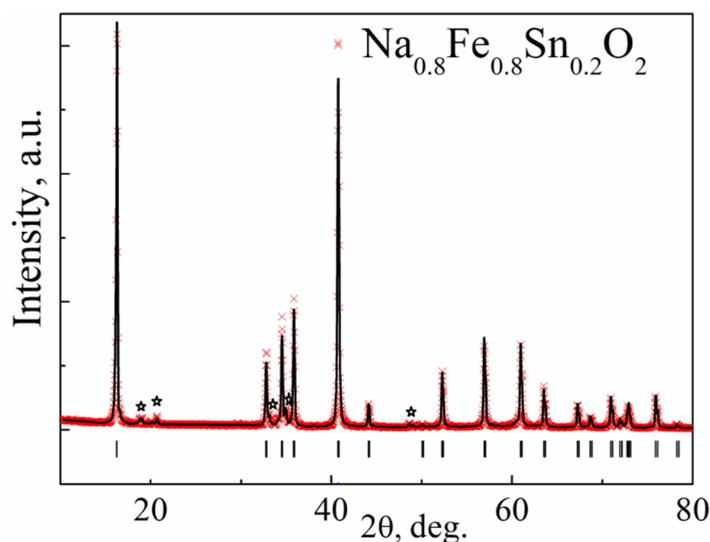
**Figure 4.** The result of the Rietveld refinement of the X-ray diffraction pattern of  $\text{Na}_{0.8}\text{Fe}_{0.8}\text{Sn}_{0.2}\text{O}_2$ . The experimental profile is represented by the red symbols (×), while the calculated profile is represented by the black line. Vertical bars denote Bragg peak positions of the main rhombohedral phase (PDF2-20-1115). Asterisks mark (☆) the monoclinic impurity phase, as it was reported in Reference [37].
