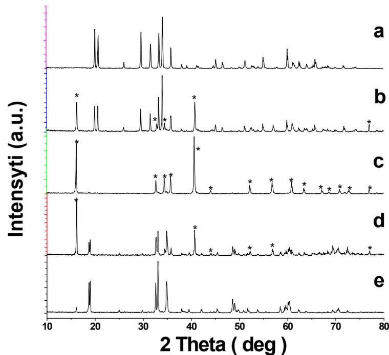
**Figure 1.** Powder XRD patterns for the samples of the NaFeO<sub>2</sub>—SnO<sub>2</sub> system: (a) NaFeO<sub>2</sub>; (b) 5; (c) 20; (d) 35 mol.% SnO<sub>2</sub>; (e) NaFeSnO<sub>4</sub>. \* Designates the lines for the phases with a rhombohedral structure.
