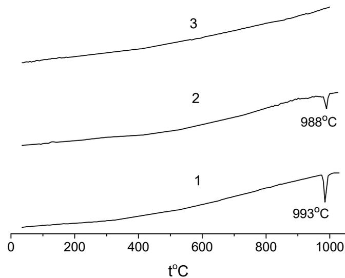
**Figure 3.** DSC curves for samples of the  $\text{NaFeO}_2$ – $\text{SnO}_2$  system: (1) 5; (2) 10; (3) 20 mol.%  $\text{SnO}_2$ .
