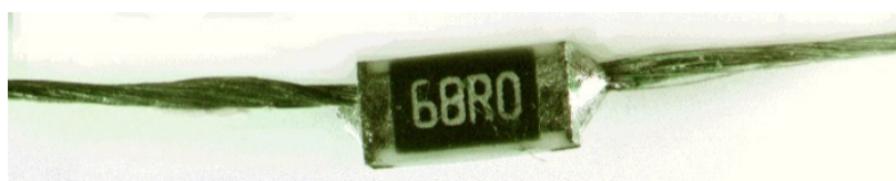
Figure 4. SMD integrated E-yarn.
