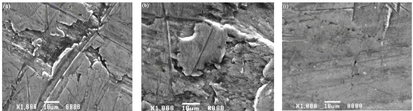
Figure 14. SEM images of (a) AA6061, (b) AA8011, (c) and weld region specimens after submersion testing in HCl .
