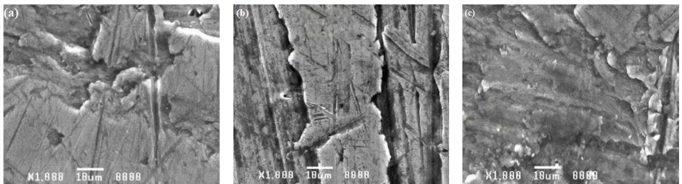
Figure 13. SEM images of (a) AA6061, (b) AA8011, (c) and weld region specimens after submersion testing in H_2SO_4 .
