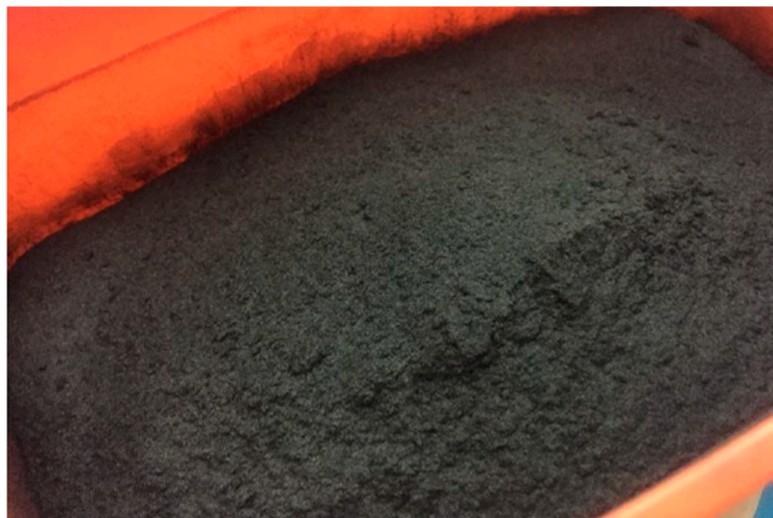
Figure 1. rCF recovered from a pyrolysis process.
