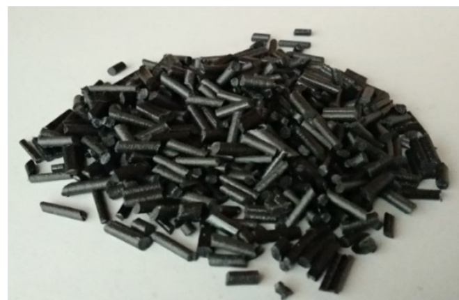
Figure 3. rCF/PLA pellets after the mixing and palletizing process.
