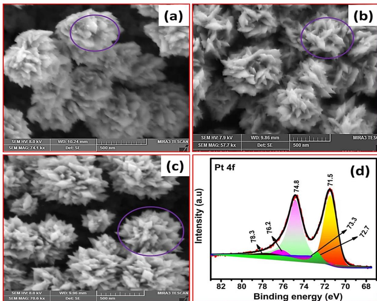
**Figure 3.** (a–c) FE-SEM micrographs for Pt structure deposited on a carbon substrate with the effect of time (300, 600, and 900 s) and (d) XPS spectrum of Pt 4f binding energy orbital with the effect of 900 s. (a–c—circled region shows flower-like morphology)
