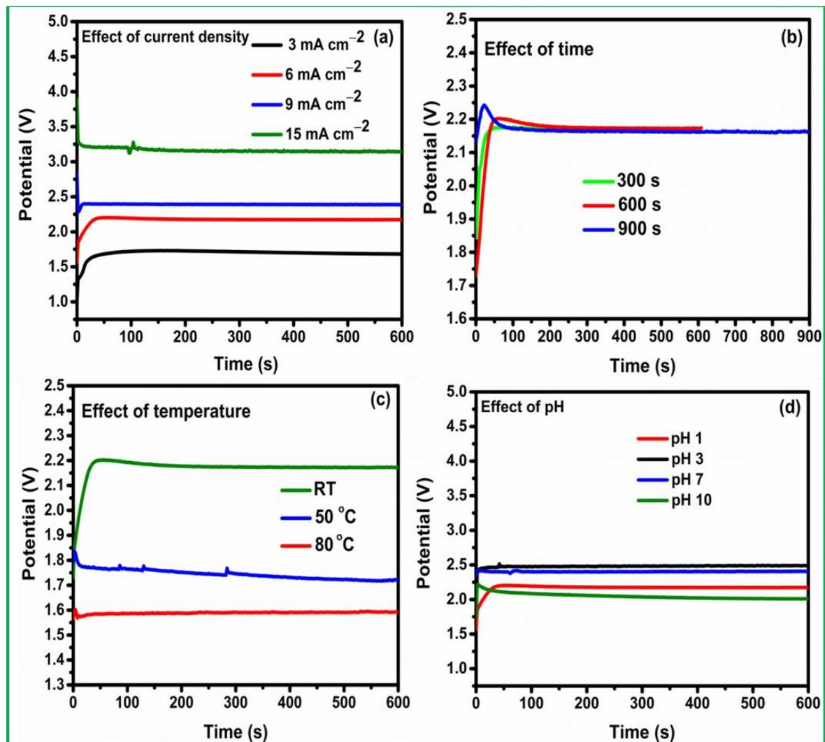
**Figure 6.** Pt deposition on a carbon surface via the (a) effect of current density, (b) effect of time (constant current density), (c) effect of temperature, and (d) effect of pH with constant current density ( $6 \text{ mA cm}^{-2}$ ).
