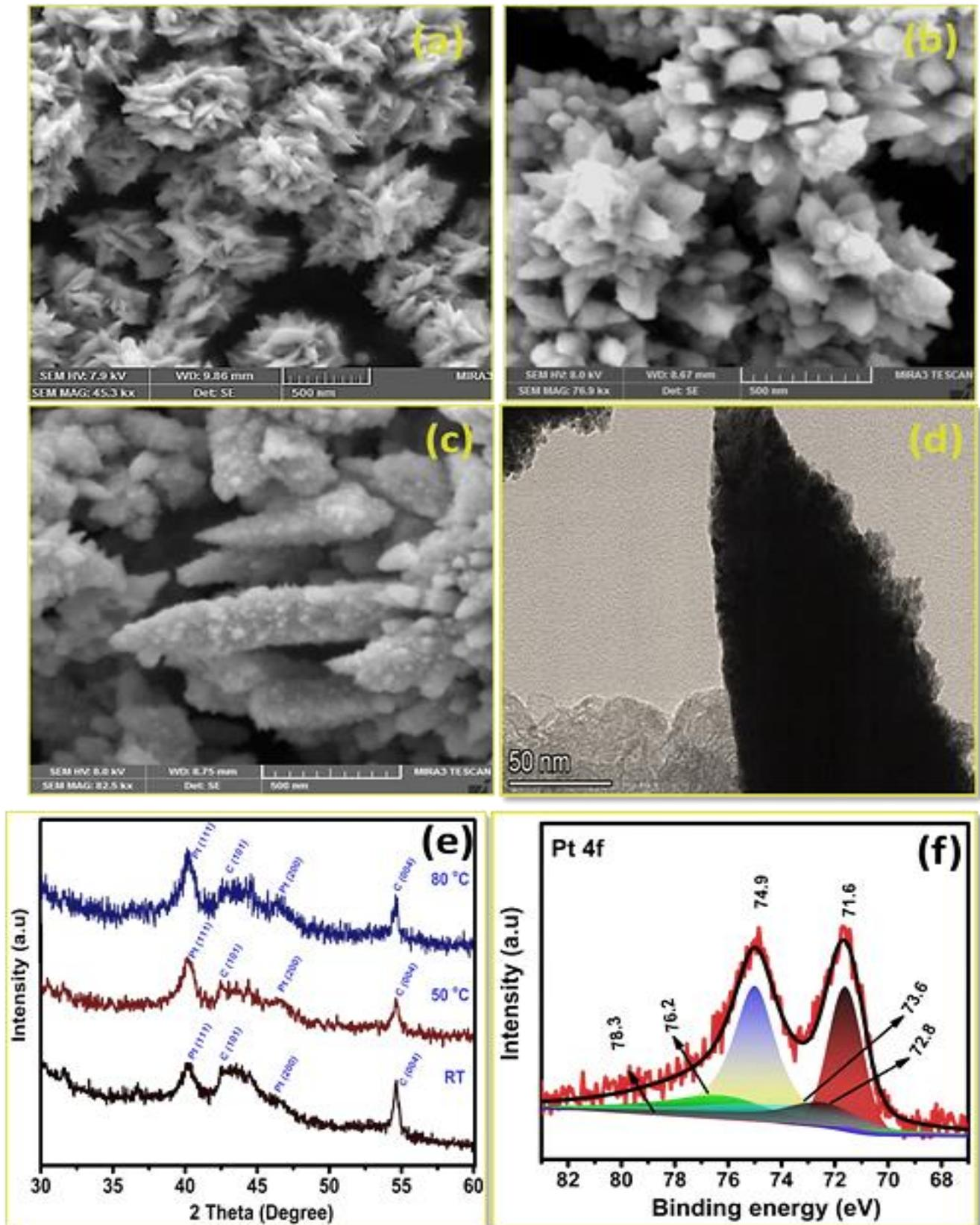
**Figure 4.** FE-SEM micrographs of Pt deposited on carbon substrate with effect of bath temperature; (a) room temperature, (b) 50 °C, (c) 80 °C, (d) HR-TEM image of Pt deposition (80 °C), (e) XRD pattern, and (f) XPS Pt 4f spectrum of Pt deposition at (80 °C).
