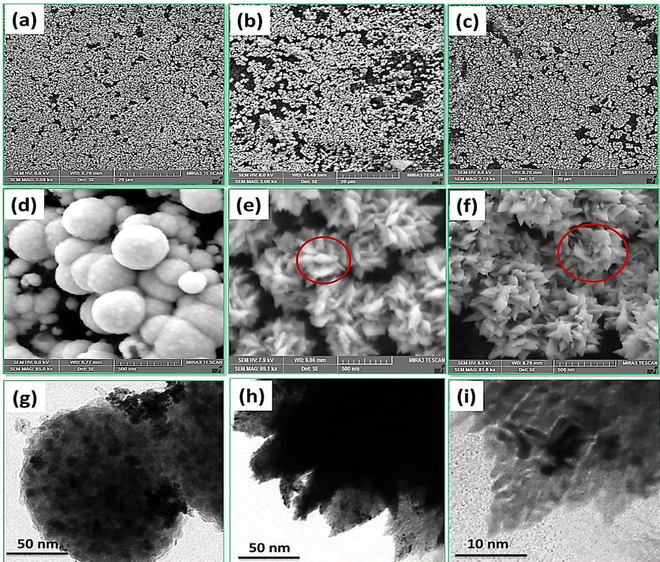
**Figure 1.** Low-magnification field emission scanning electron microscope (FE-SEM) micrographs (a–c) and high magnification (d–f) with various Pt deposition current densities of 1.5, 6, and 15 mA cm<sup>-2</sup> and (g–i) high resolution transmission electron microscopy (HR-TEM) image with Pt deposition current densities of 1.5 and 6 mA cm<sup>-2</sup>. (e,f—circled region shows dendritic flower-like morphology)
