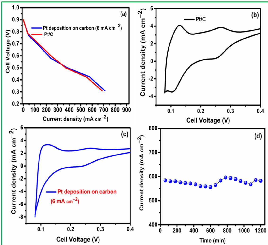
**Figure 7.** (a) Fuel cell performance, (b,c) H<sub>2</sub> adsorption and desorption behaviour of Pt/C and Pt deposited on carbon (6 mA cm<sup>-2</sup>), and (d) stability test at 0.4 V for Pt deposited on carbon (6 mA cm<sup>-2</sup>).
