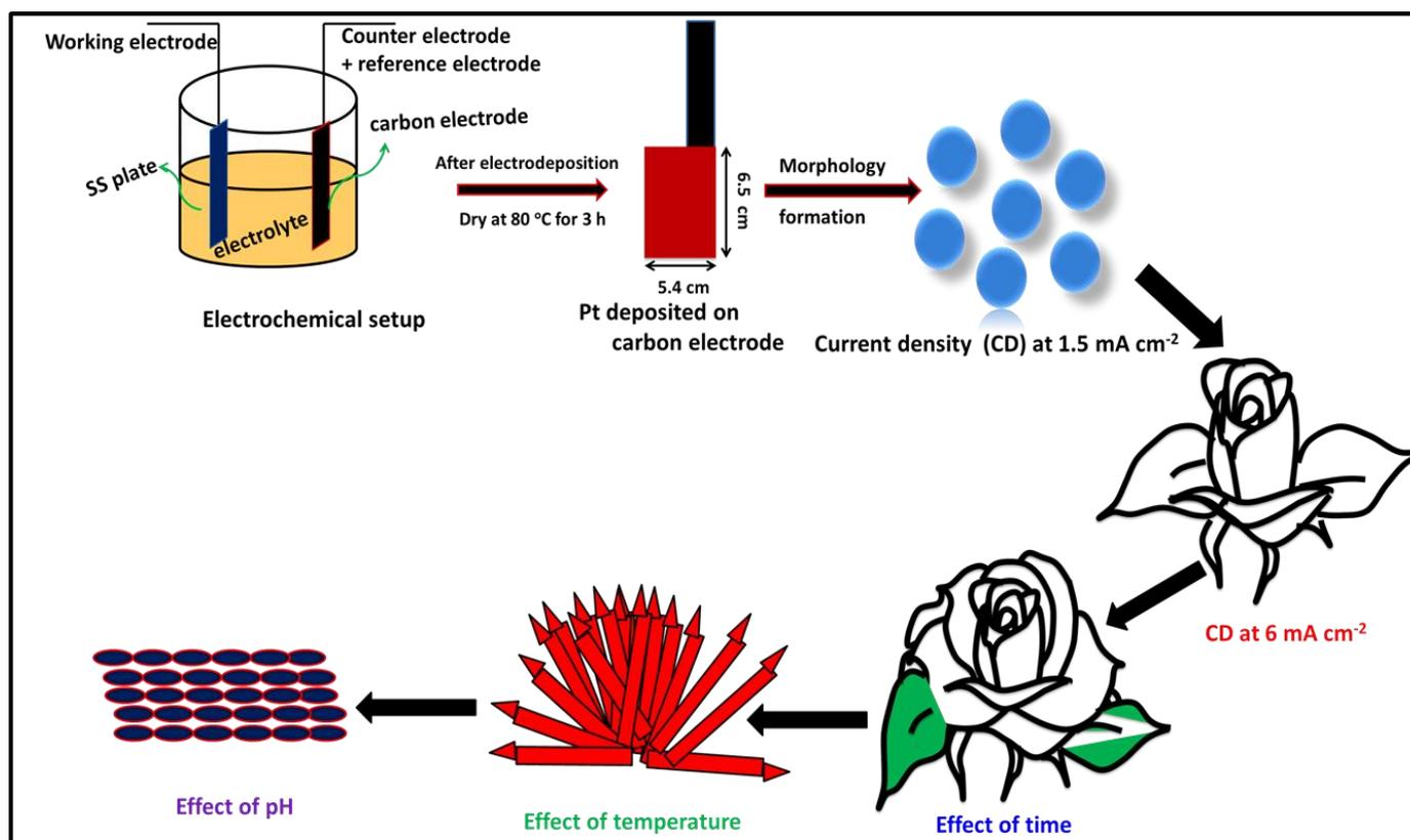
**Scheme 1.** Schematic diagram of electrochemical two electrode systems and formulated electrolyte with exposed conductive carbon substrate (5.4 cm × 6.5 cm) and proposed Pt morphology.
