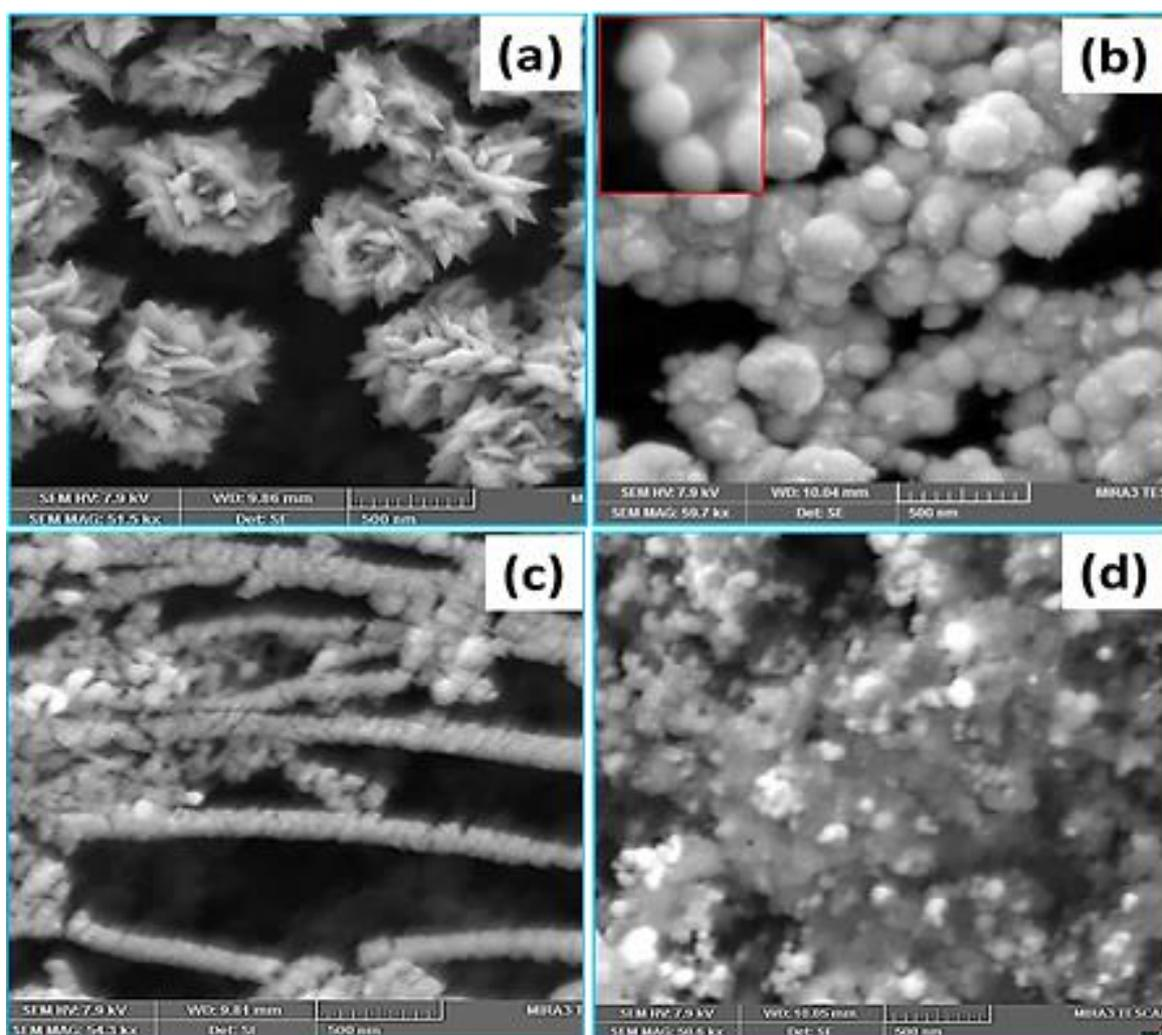
**Figure 5.** FE-SEM images of Pt deposited with influence of pH: (a) pH 1, (b) pH 3, (c) pH 7, and (d) pH 10. (b—inset shows pellet-shaped globular morphology of deposited Pt)
