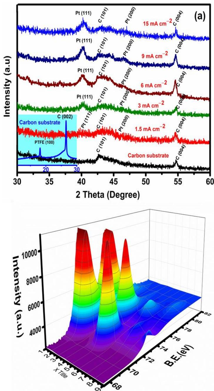
**Figure 2.** (a) Typical X-ray diffraction (XRD) pattern with Pt deposition of different current densities on a carbon substrate. (Note: The expended region between 10° and 30° indicated two different peaks due to carbon and PTFE observed for all samples). (b) 3D view XPS spectrum of Pt 4f binding energy orbital.
