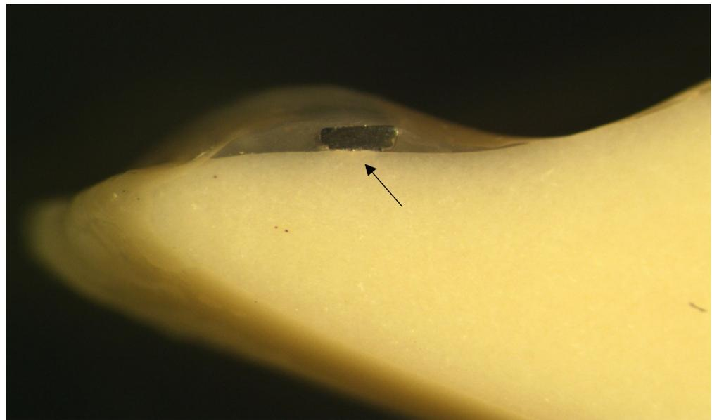
**Figure 4.** Photograph of the longitudinal section of a Frasaco tooth Straight 8 and flowable resin composite cover. The arrow points the place of the retainer.
