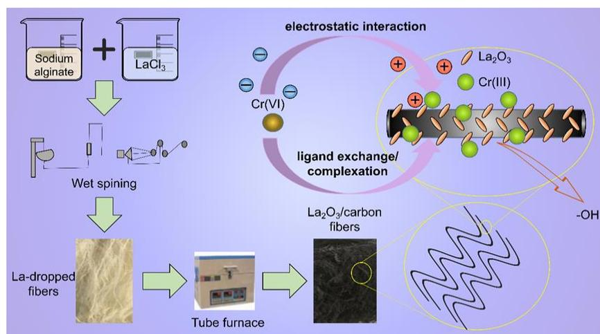
**Figure 10.** Preparation process of La-BC and the mechanism of Cr (VI) adsorption with it.
