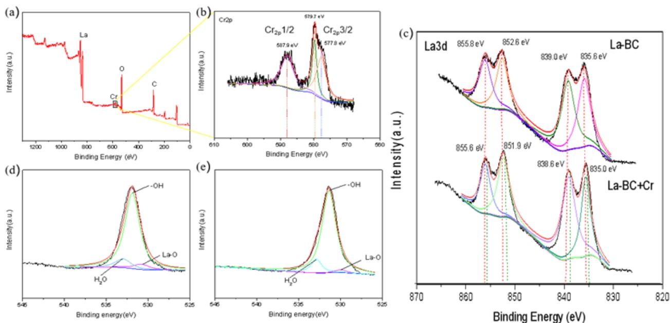
**Figure 9.** (a) XPS spectra of the La-BC (900 °C) after Cr (VI) adsorption(a); (b) Cr2p; (c) La3d; (d) the O1s spectra of La-BC (900 °C) before and (e) after Cr (VI) adsorption.
