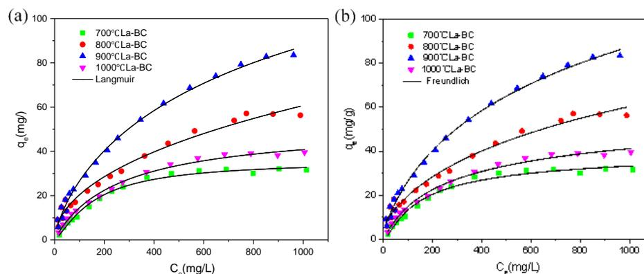
**Figure 5.** Fitting the adsorption data of Cr (VI) on La-BC (900 °C) to (a) the Langmuir isotherm, and (b) the Freundlich isotherm.
