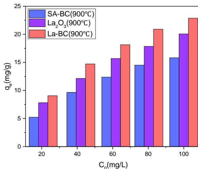
**Figure 1.** Pre-experiment: comparison of the adsorption capacity of Cr (VI) by SA-BC, La<sub>2</sub>O<sub>3</sub> and La-BC.
