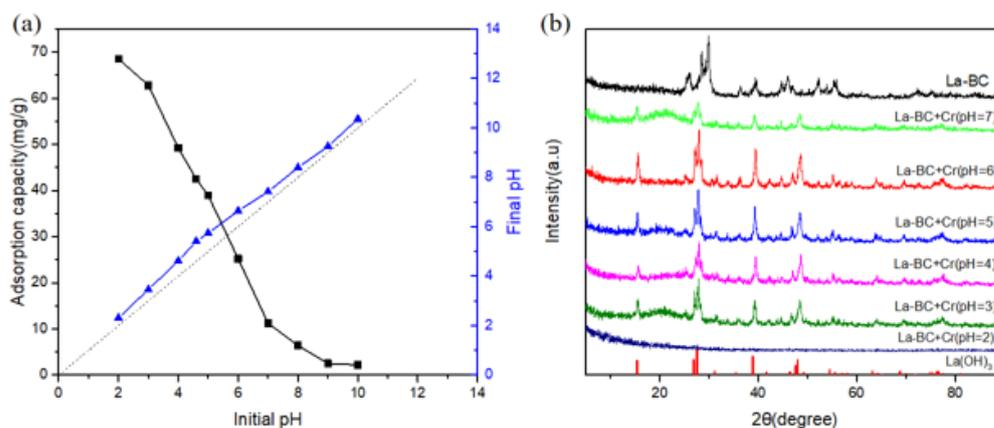
**Figure 7.** (a) The effect of pH on the adsorption amount, and the comparison of the initial and final pH; (b) the XRD images of La-BC (900 °C) after the adsorption with a pH range of 2–7.
