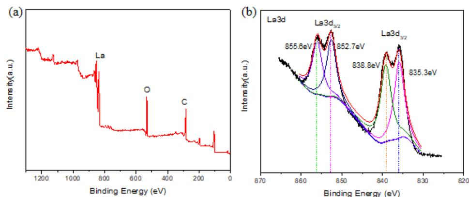
**Figure 4.** (a) XPS spectra of the La-BC (900 °C) before Cr (VI) adsorption; (b) La 3d spectra of La-BC (900 °C) before Cr (VI) adsorption.
