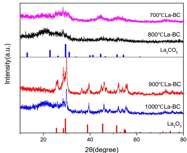
**Figure 3.** XRD patterns of the different carbonization temperatures of the La-BC samples.
