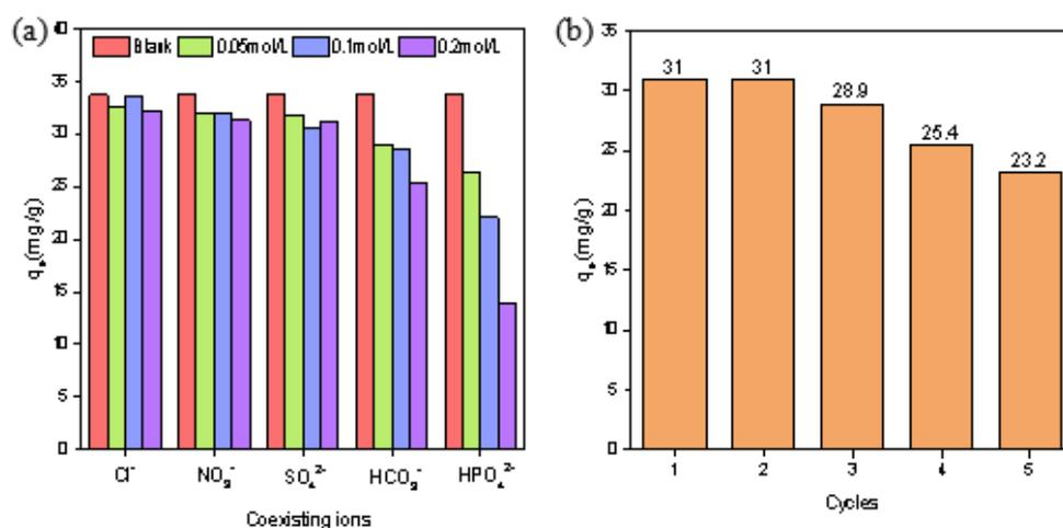
**Figure 8.** (a) Effect of coexisting ions on the adsorption amount of Cr (VI); (b) five cycles of Cr (VI) adsorption by La-BC (900 °C).
