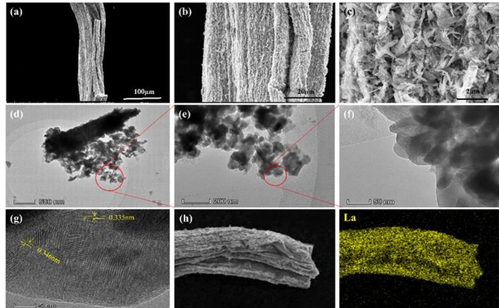
**Figure 2.** (a–c) SEM images of La-BC; (d–g) TEM images of La-BC; (h) elemental mapping images of La-BC.
