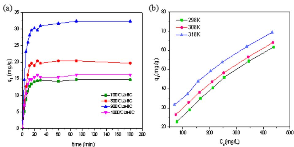
**Figure 6.** (a) Relationship between the adsorption amount of Cr (VI) and the adsorption time by La-BC at four carbonization temperatures; (b) relationship between the adsorption amount of Cr (VI) and the adsorption temperature by La-BC (900 °C).
