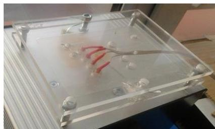
**Figure 5.** The photo of construction with four electrodes for the measurement of electrical resistance of textiles by the four-point method.
