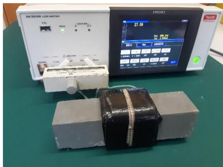
**Figure 11.** The setup for measuring 40 mm × 40 mm × 160 mm specimens.
