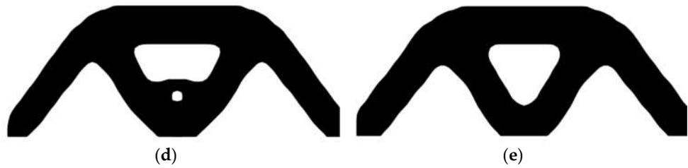
**Figure 17.** Optimal design problem of simple bridge beam by CBT level set topology optimization, (a) initial shape; (b) iteration 10; (c) iteration 20; (d) iteration 40; (e) optimized shape.
