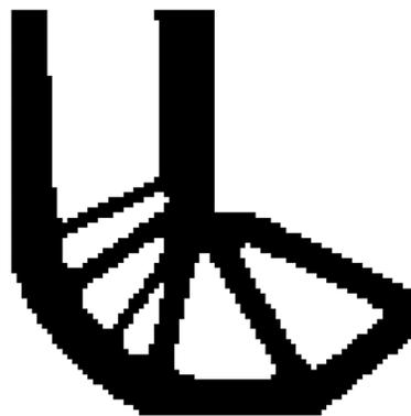
Figure 10. Optimized shape of L-shaped by traditional BESO.
