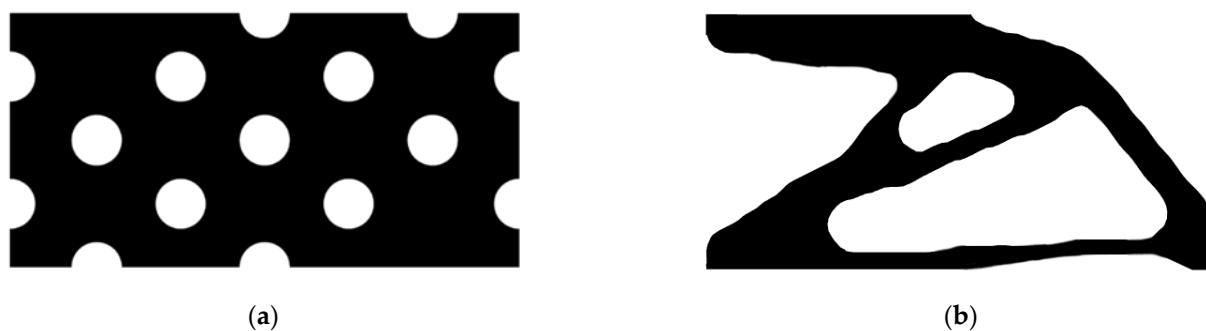
Figure 23. Optimal design problem of cantilever beam by classical level set topology optimization, (a) initial shape; (b) optimized shape.
