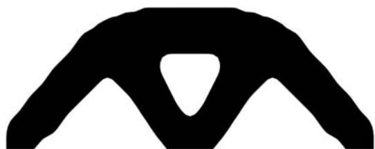
Figure 20. Optimized shape of simple bridge beam with a volume fraction of 0.75.
