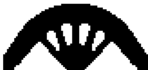
Figure 7. Optimized shape of simple bridge beam by the improved method.
