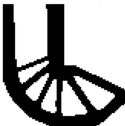
Figure 12. Optimized shape of L-shaped by the improved method.
