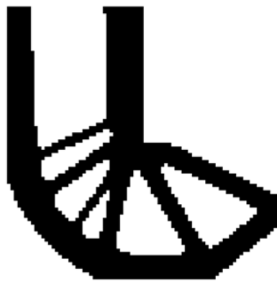
Figure 10. Optimized shape of L-shaped by traditional BESO.
