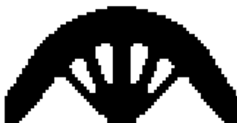
Figure 5. Optimized shape of simple bridge beam by traditional BESO.
