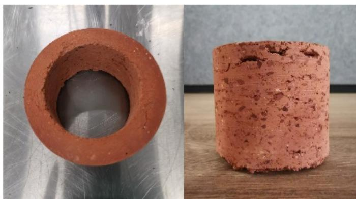
**Figure 1.** The core of the brick extracted for CHNS analysis.
