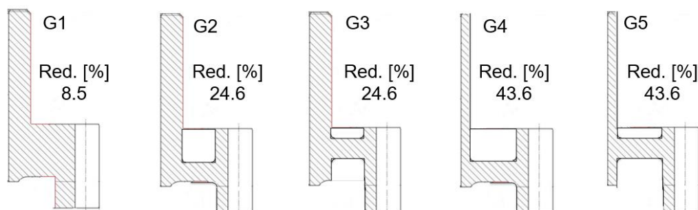
Figure 2. Geometry variations G1–G5 and percentage of mass reduction achieved.
