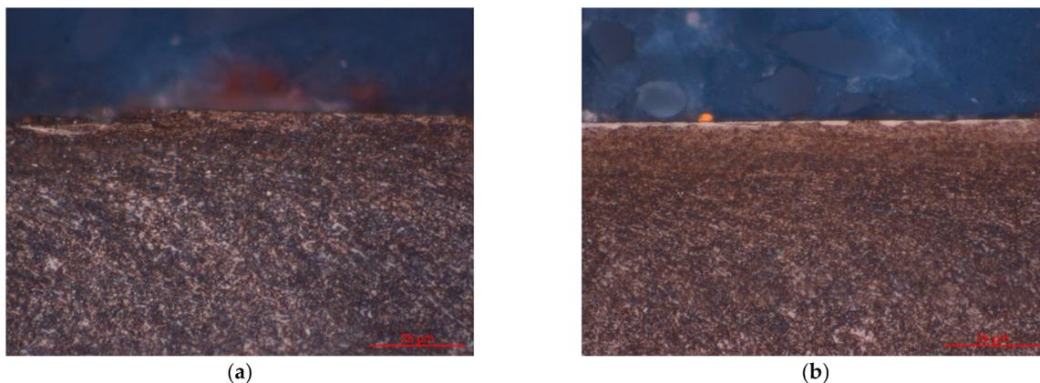
**Figure 11.** Optical observations on the cross-section of: (a) 343 °C austempered disks, (b) 585 °C quenched-tempered disks.
