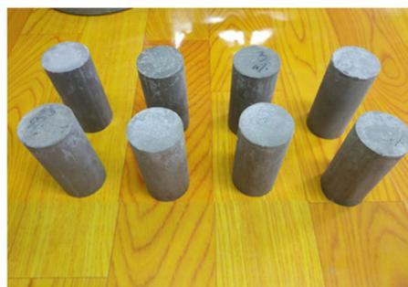
**Figure 2.** Silica fume cement stabilized soil samples after curing.
