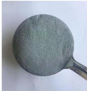
**Figure 1.** Silica fume sample particles.
