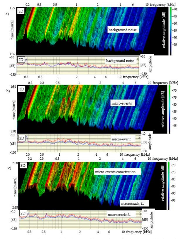
**Figure 5.** Cement paste with  $V_f = 6\%$  in the bending test and the AE, with 3D and 2D sound spectra: (a) background noise; (b) micro-events; (c) for and micro-events concentration.
