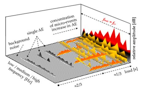
**Figure 7.** The range of micro-events in cement composites ( $f_{cr} = f_{max}$ ) identified by means of a space sound spectrum.
