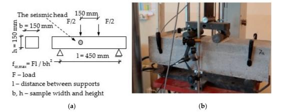
**Figure 1.** Four-point bending test: the specimen before the test in the test machine: (**a**) diagram of the test [44], (**b**) the specimen before test.
