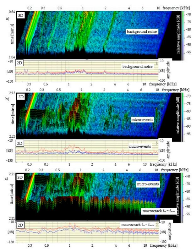
**Figure 6.** Concrete with traditional continuous reinforcement during the bending test and the AE, with 3D and 2D sound spectra: (a) background noise; (b) micro-events; (c) micro-events and macrocrack  $f_{cr} = f_{max}$ .
