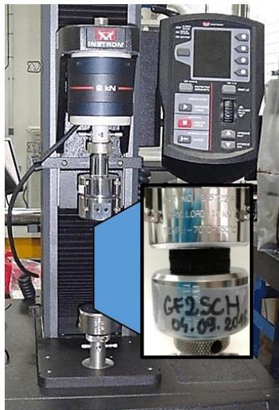
**Figure S6.** Measurement of the mechanical properties of fibrous carbons under compression using an Instron 5944 universal testing machine (INSTRON, 825 University Ave Norwood, MA, 02062-2643, USA). The insert shows the compression platens on either side of a specimen just prior to its compression.
