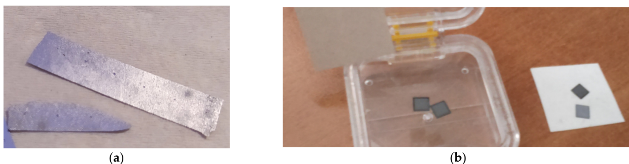
Figure 5. (a) An example of a thin diamond film grown on silicon. After the thinning of the silicon wafer up to a thickness of about 80 \mu\text{m} , substrate bending is clearly evidenced. (b) 5 mm \times 5 mm diamond on 120 \mu\text{m} thick silicon plates after membrane fabrication.
