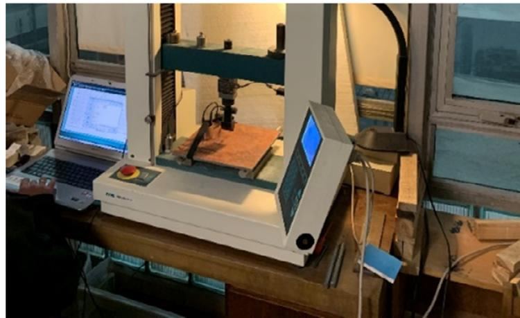
Figure 10. Three-point bending flexural testing machine.
