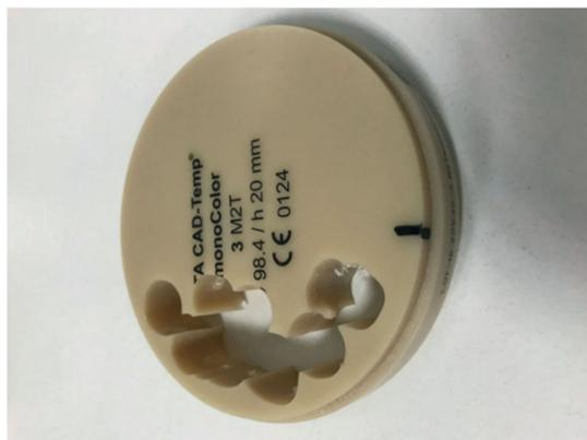
**Figure 6.** Vita CAD-Temp disk, reprinted with permission from ref. [44] (Copyright 2020 Inżynier i Fizyk Medyczny).
