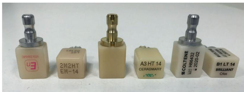
**Figure 1.** Examples of commercial CAD/CAM blocks. From the left: resin matrix composite Vita Enamic, resin matrix composite CERASMART and composite Brilliant Crios, reprinted with permission from ref. [44] (Copyright 2020 Inżynier i Fizyk Medyczny).
