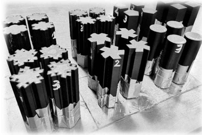
**Figure 2.** Cast concrete–plastic specimens.
