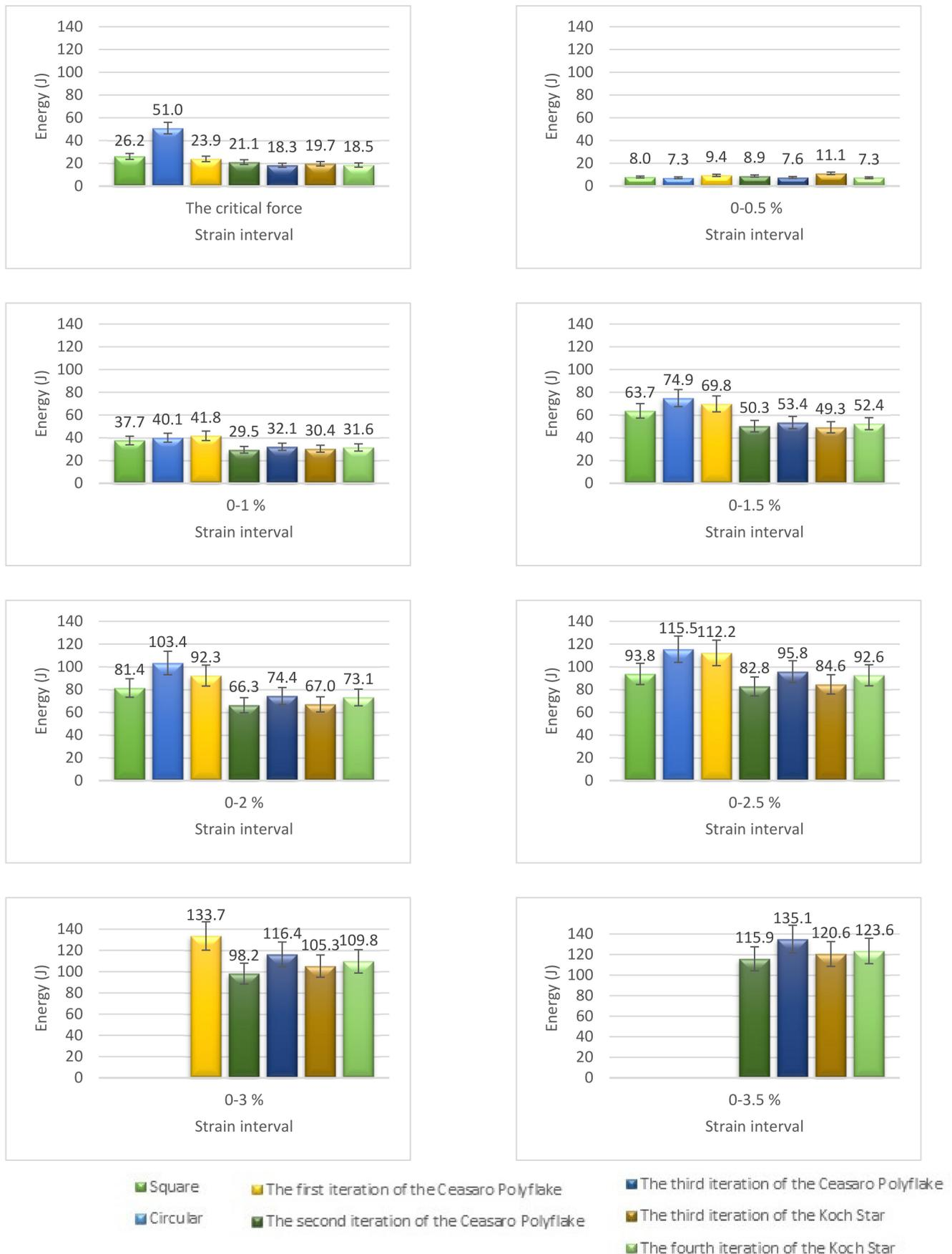
Figure 9. The energy needed to achieve a particular strain of tested concrete-plastic columns.
